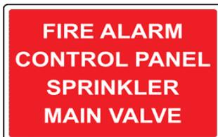
If the sprinkler riser/control valve and fire alarm control panel are in the same room, the sign should read “FIRE ALARM & SPRINKLER CONTROL ROOM” or “FACP & SPRINKLER CONTROL ROOM” be provided which consist of 7" high by 10" width with a 0.5" letter stroke white reflective letters on a red background, and shall be permanently attached, at normal eye level to the door leading to the fire sprinkler control equipment unless otherwise approved by the Office of the Fire Marshal.
