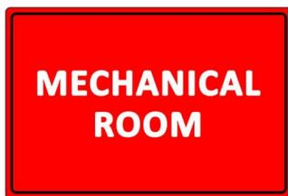
Doors into Mechanical Equipment rooms shall be provided with a plainly visible and legible sign stating MECHANICAL ROOM which consist of 7" high by 10" width with a 0.5" letter stroke white reflective letters on a red background, and shall be permanently attached, at normal eye level to the door leading to the fire pump equipment unless otherwise approved by the Office of the Fire Marshal
